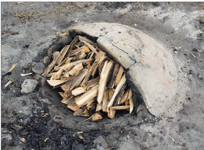
Fig. 5. Filling of the inside of the pit and dome with pine stumpwood (photo by K. Wasilczyk).
