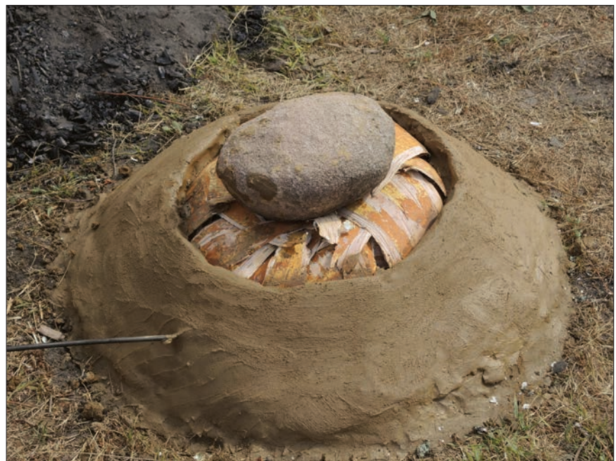
Fig. 2. Wood tar earthen pit during the filling and building of the dome (photo by K. Wasilczyk).
